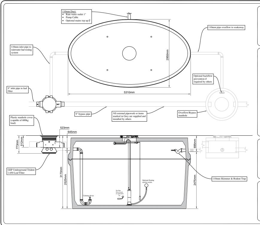
Tank lifting limitations: Max chain angle < 60°
