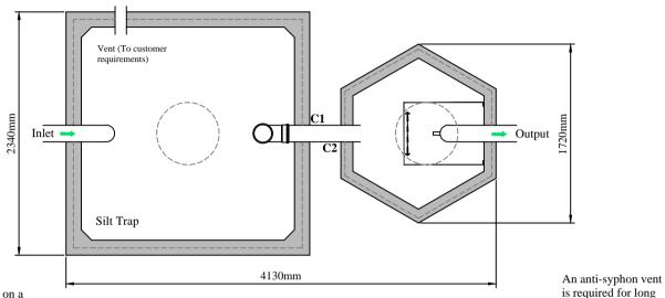
All the tanks must be placed on a perfectly level and firm suitable base.
