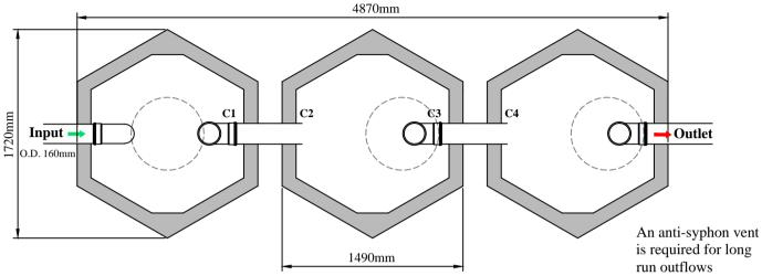
All the tanks must be placed on a perfectly level and firm suitable base.
