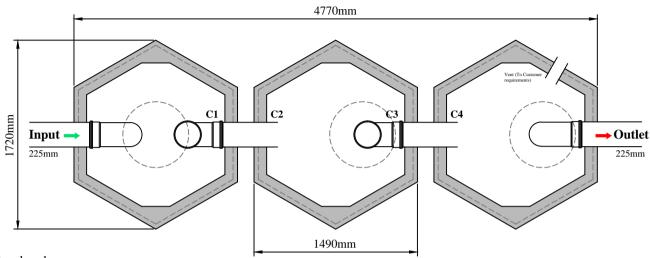
All the tanks must be placed on a perfectly level and firm suitable base.
