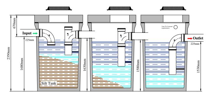
20 l/s flow 1,110m sq. coverage 1,500 lit. emergency oil retention 2,300 lit. silt capacity
